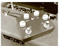
You have three gain stages – an input and an output stage, and between those two you generate the boost. You set the Gain at the first stage with the control. That goes to the output gain
