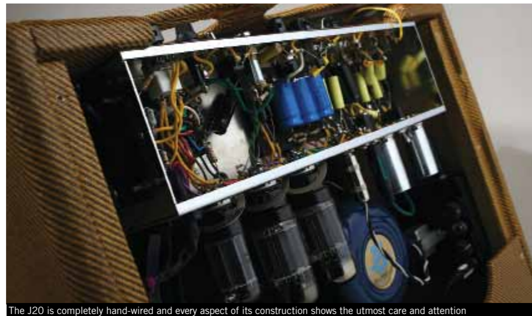
The J20 is completely hand-wired and every aspect of its construction shows the utmost care and attention
