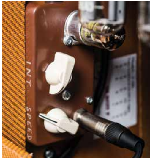
Optional tremolo and reverb modules are mounted around the back but footswitchable on the fly
